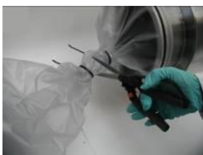
Fig 18. Camfil Bag Welding Method (Weld, Cut and Separation).
