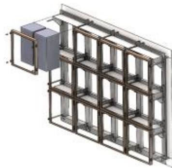
Fig 3. 1960's Non Safe Change Housing In Exclusion Area.
