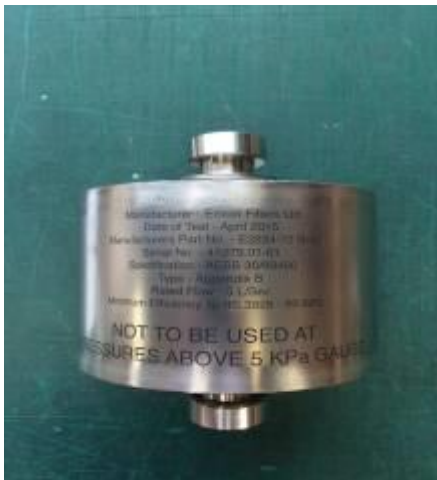
Fig 19 Picture shows a 5Ltr/s Process HEPA Filter
