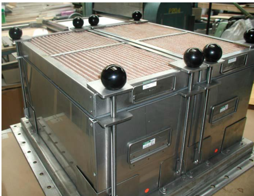
Fig 20. Split 609 x 609 unit for “Safe” Intermediate Level Waste disposal (fitted with split pre-filters).
