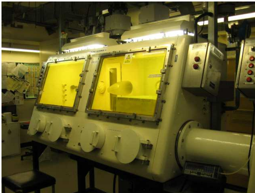
Photo B1. Typical Small Glovebox
