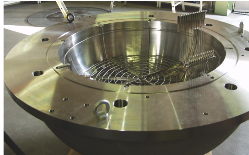
Fig. 4. Scaled RPV experimental vessel [2, 3].
