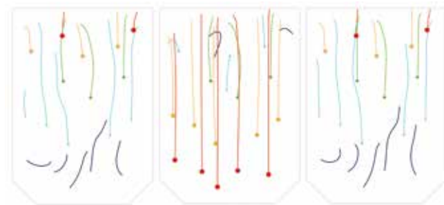
FIGURE 8: Bubble paths over 60 seconds for the base case (left), the bubble size sensitivity where the bubble positions were reversed (middle), and the drag coefficient sensitivity study where a UDF was used to account for reduced tangential shear stress (right).
