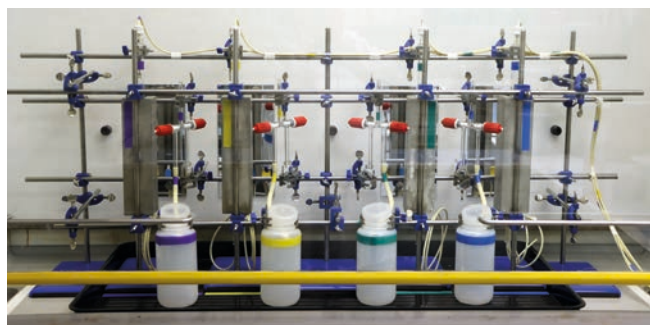
Figure 4. Ion exchange rig based on four individual "Thorium Cows" used for the recovery of ^{228}\text{Th} , ^{224}\text{Ra} , ^{212}\text{Pb} and ^{212}\text{Bi}
