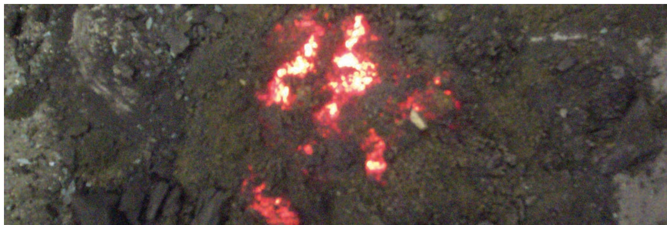
Figure 1: Bulk \text{UH}_3 self-heating
