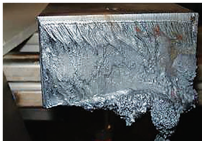
Figure 3: 100mm steel cut using 8kW laser with air-cooled cutting head; CEA, France
