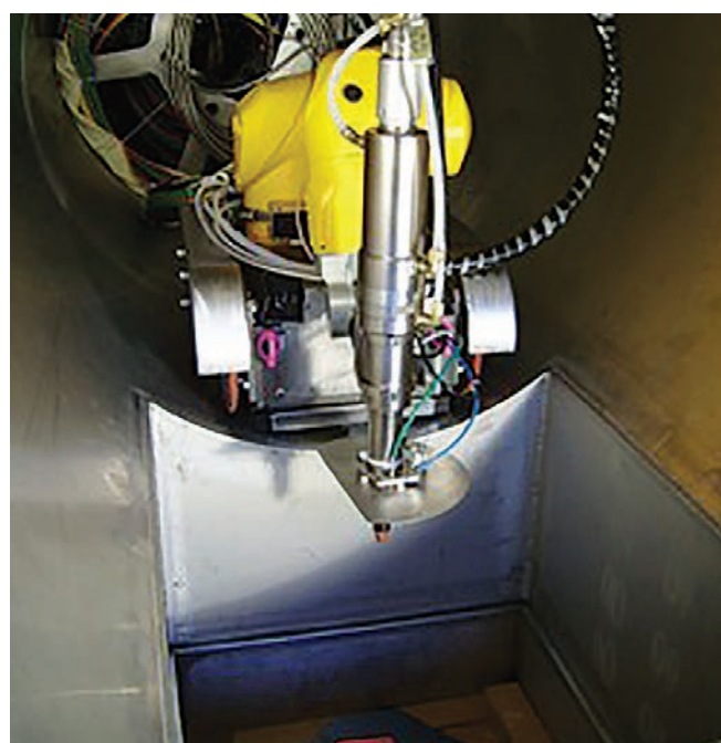
Figure 4: Laser module mounted on the remotely operated vehicle (courtesy of Areva)
