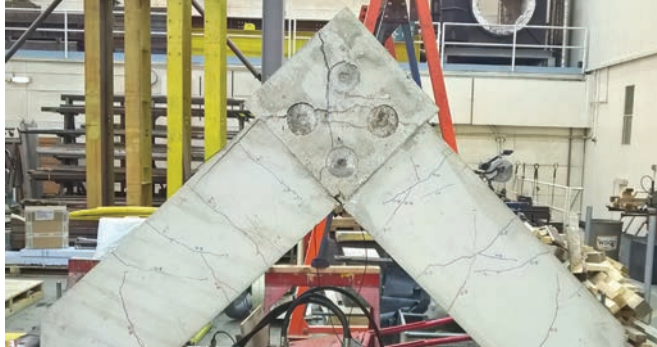
Figure 9: A headed bar corner joint ready for destructive testing at the Building Research Establishment.
