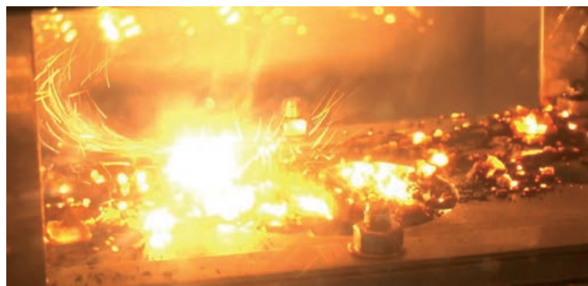
Figure 3: Transient violent reaction of UH 3 in air
