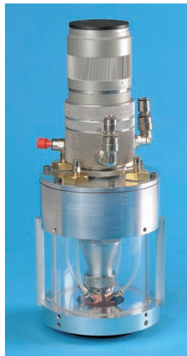
Figure 1: Underwater laser cutting head design (left) and final designed module (right); TWI
