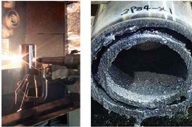
Figure 5: Laser cutting of double skin pipe using 8kW, with 4mm thick pipe cut at speeds of 150mm/min
