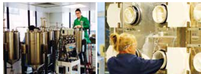
FIGURE 5: New skills and capabilities developed by the programme – (left) the engineering scale centrifugal contactor rig at the University of Leeds and (right) plutonium glove box training at NNL.
