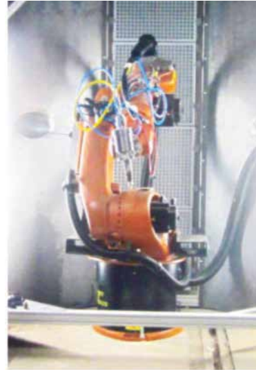
FIGURE 5: Alpha glovebox laser cutting robot
