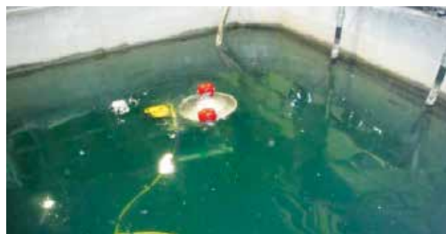
FIGURE 7: Inactive trial of closed-loop variable buoyancy lifting system at NNL's Workington laboratory
