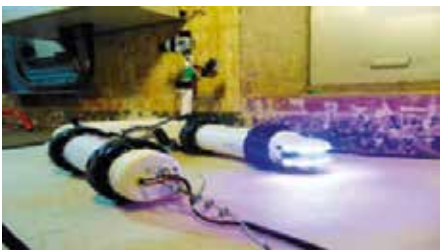
FIGURE 4: MIRRAX Alpha glovebox decommissioning
