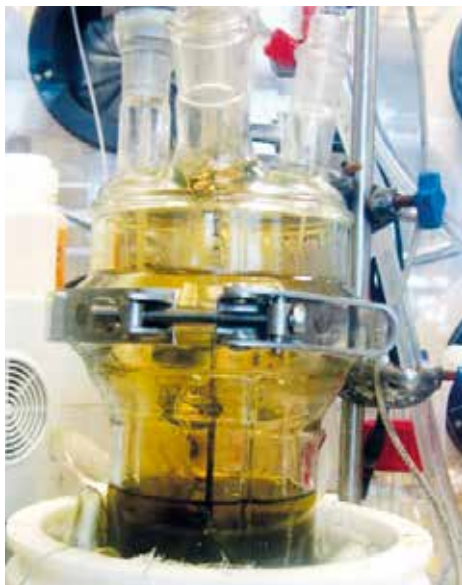
FIGURE 3: MOX pellet dissolution in NNL's PuMA Lab
