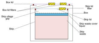
FIGURE 3: Schematic of the ILW skip
