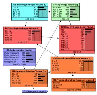
FIGURE 6: Quantified Bayesian network for uncertainty analysis of hydrogen concentration in ILW skip (continuation from Figure 5 node F3)
