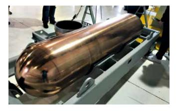
FIGURE 2: NWMO's Mk II canister
