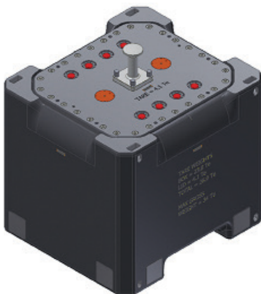
Figure 2: Self-shielded box concept (Sellafield Ltd, 2017)
