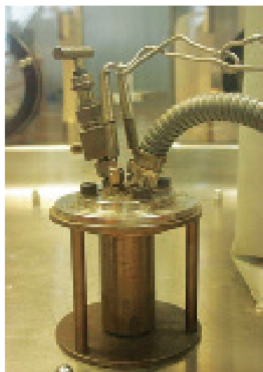
Figure 10: Baskerville Reactor (top left) used for pressure-temperature measurements of \text{PuO}_2 water adsorption-desorption experiments and the associated glove box furnace for heating the reactor (top right). Also shown are examples of the measured variation of water sorption with relative humidity for a range of specific surface areas (bottom)
