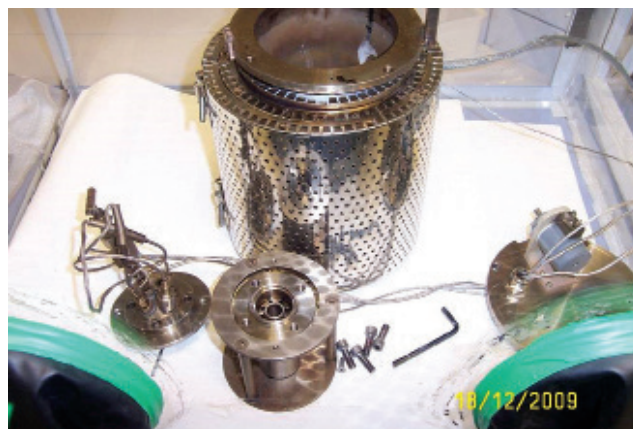
Figure 10: Baskerville Reactor (top left) used for pressure-temperature measurements of \text{PuO}_2 water adsorption-desorption experiments and the associated glove box furnace for heating the reactor (top right). Also shown are examples of the measured variation of water sorption with relative humidity for a range of specific surface areas (bottom)
