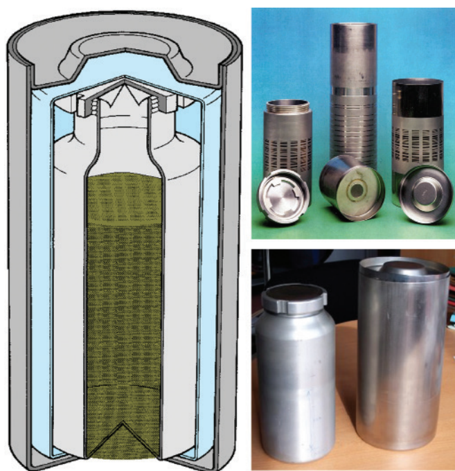
Figure 1: Multiple barrier containment \text{PuO}_2 storage cans. Clockwise from top right are containers for Thorpe \text{PuO}_2 , Magnox \text{PuO}_2 and a cutaway diagram of the assembled Magnox package
